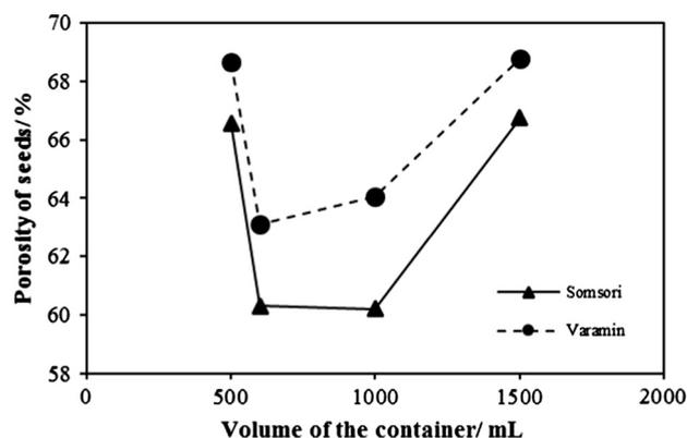
**Figure 4** Effect of the volume of the container on porosity of melon seeds.
