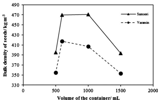
**Figure 2** Effect of the volume of the container on bulk density of melon seeds.
